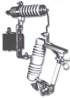
Over the arm mounted, 15KV Type C cutout, direct connected, 9/10kV arresters, with crossarm mounting bracket.
