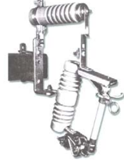
Over the arm mounted, 15KV Type C cutout, external gap, 9/10KV arresters, on crossarm bracket.
